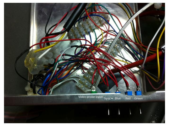
Essentially, this modification allows you to replace the green drive to the monitor with a signal of your choice - that from the JAMMA connector, or wherever you're placing your probe.
