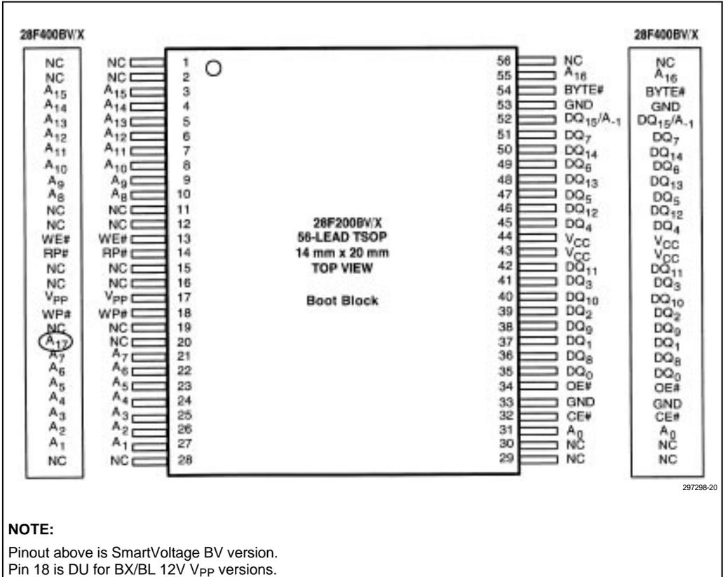
**Figure 2-13. The 56-Lead TSOP Pinout for 28F200BV and BX, and 28F400BV and BX**
