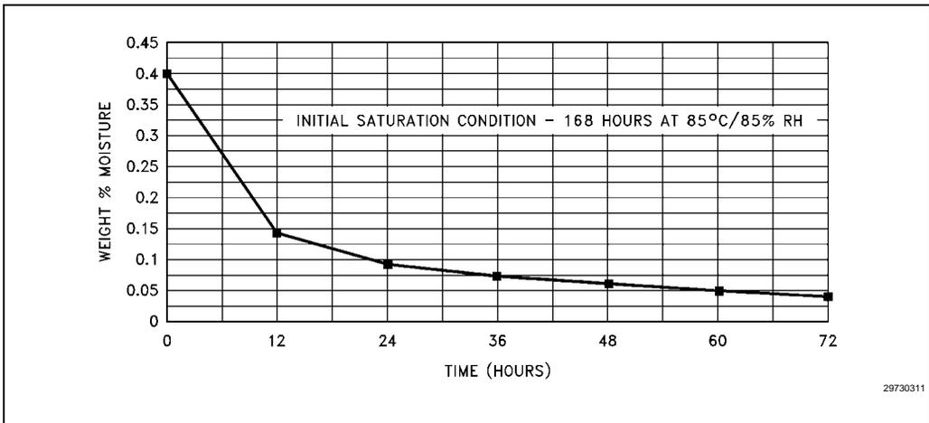
Figure 7-18. 68-Lead PLCC Desorption at 125 °C
