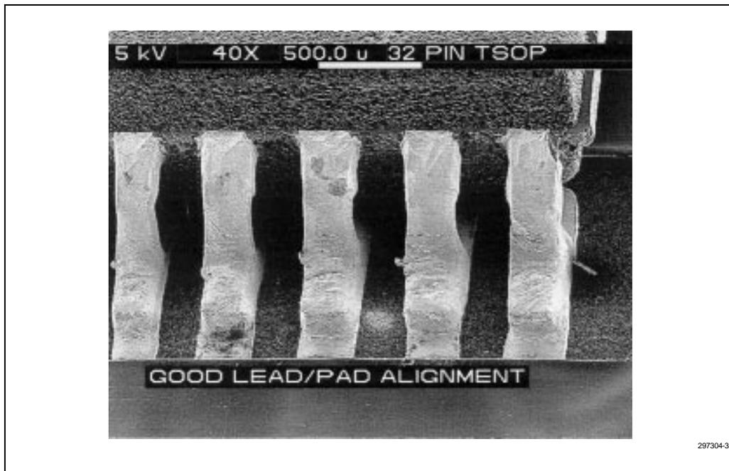
Figure 8-3. Example of Good Placement
