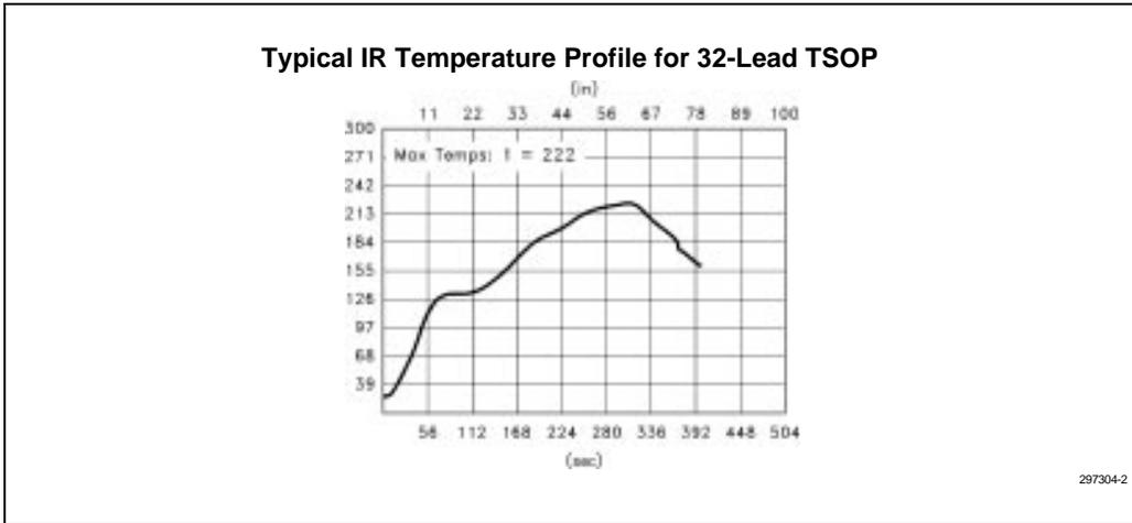
**Figure 8-2. IR Characteristics Typical Profile**
