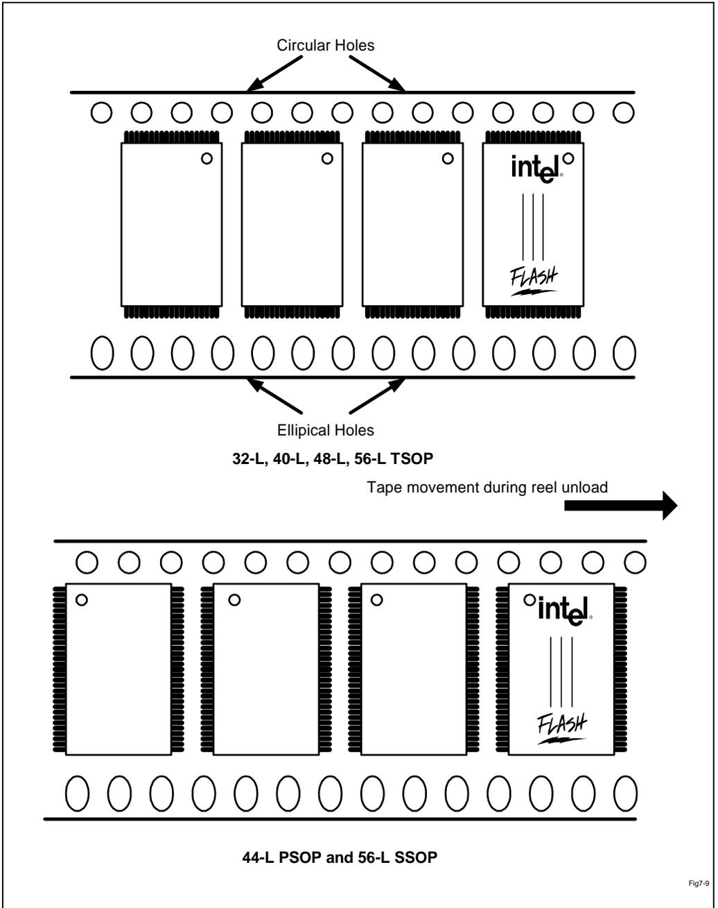
Figure 7-8. SOP Tape and Reel Orientation
