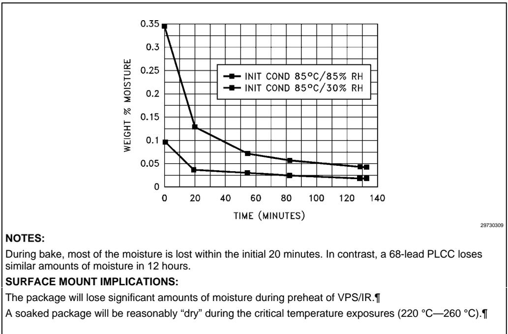
Figure 7-16. TSOP Moisture Desorption at 125 °C
