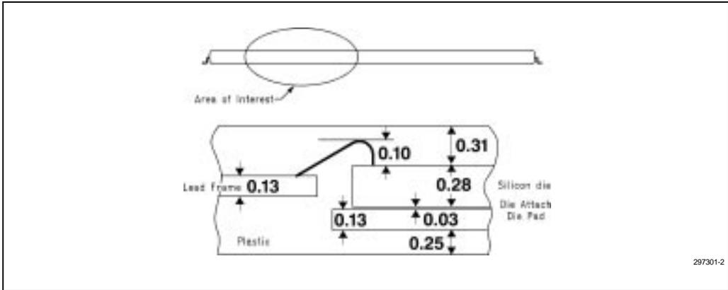
Figure 5-2. Typical TSOP Cross Section
