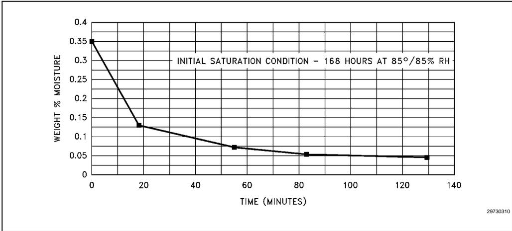
Figure 7-17. TSOP Desorption at 125 °C
