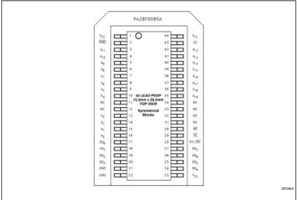
Figure 2-11. 44-Lead PSOP Package Pinout for 28F008SA
