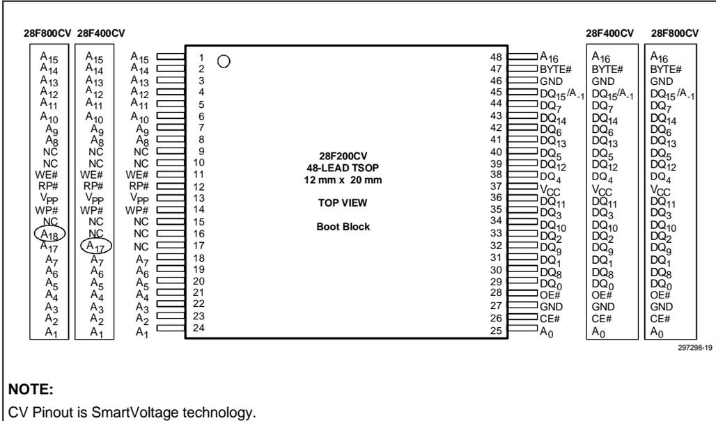
Figure 2-12. The 48-Lead TSOP Pinout for 28F200CV, 28F400CV and 28F800CV
