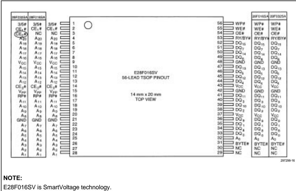
**Figure 2-14. 28F016SV 56-Lead TSOP Pinout Configuration Shows Compatibility with 28F016SA/28F032SA**
