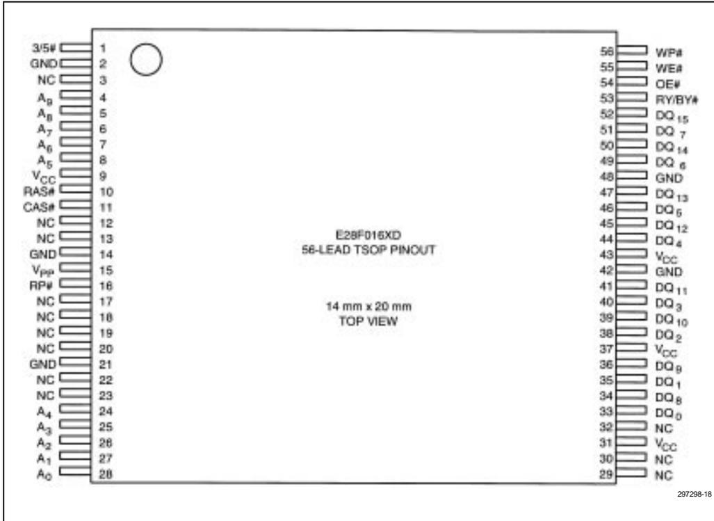
Figure 2-16. 28F016XD 56-Lead TSOP Type I Pinout Configuration
