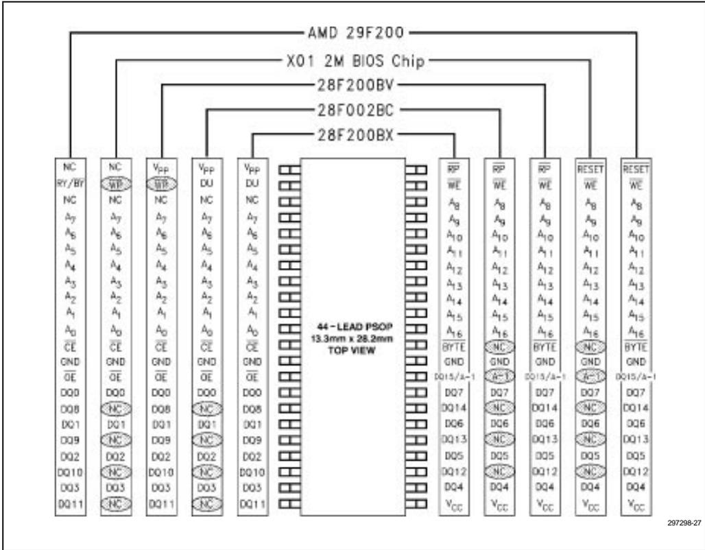
Figure 2-8. The 44-Lead PSOP Pinout for X01 2M BIOS Chip, 28F200BV, 28F002BC, 28F200BX vs. AMD 29F200
