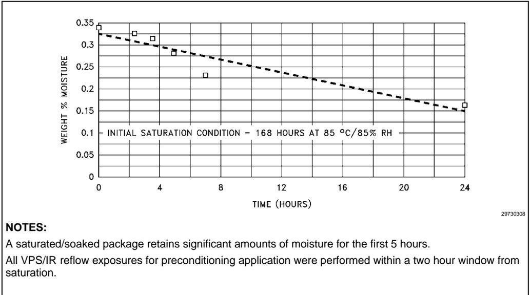
Figure 7-15. TSOP Moisture Desorption at 25 °C
