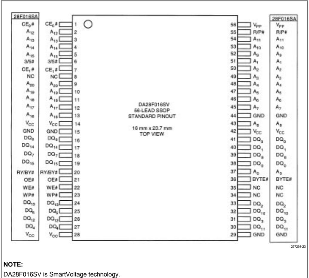
Figure 2-17. 56-Lead SSOP Pinout Configuration
