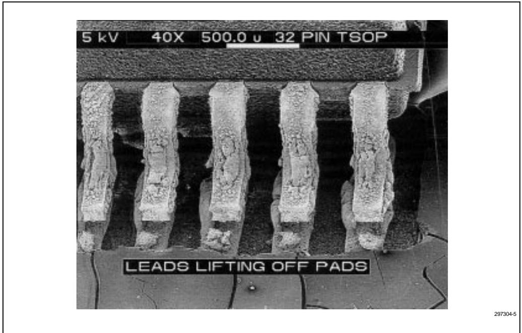
Figure 8-5. Example of Lifting
