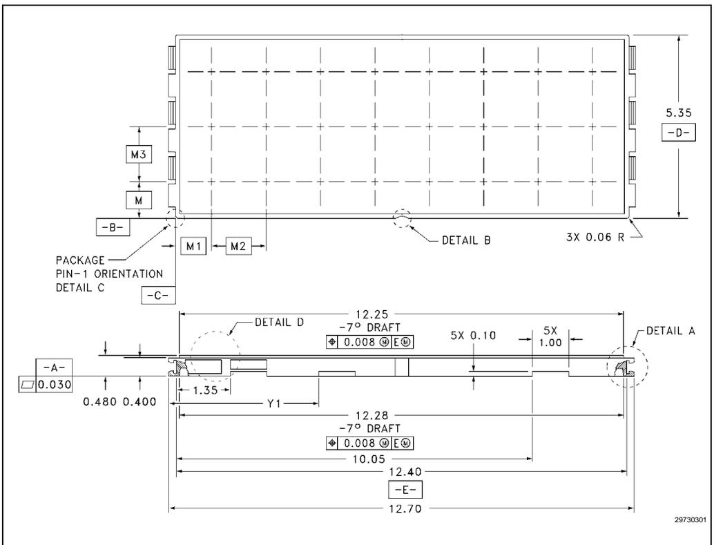
Figure 7-1. SOP Thick Tray Diagram
