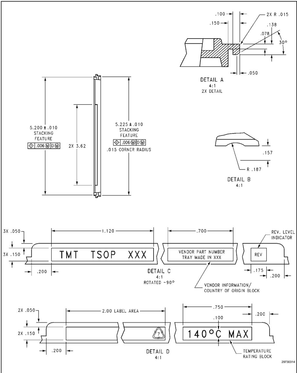
Figure 7-4. SOP Thin Tray Diagram (Detailed View)
