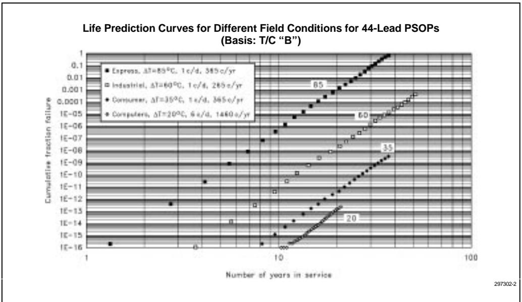
Figure 6-2. 44-Lead PSOP Life Prediction Curves
