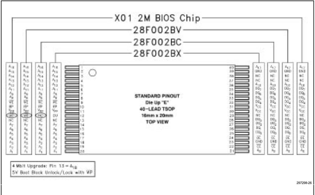
Figure 2-7. The 40-Lead TSOP Pinout for X01 2M BIOS, 28F002BV, 28F002BC, and 28F002BX
