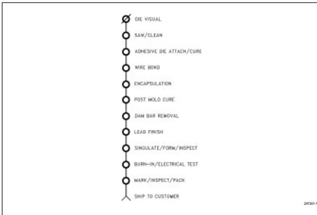
Figure 5-1. SOP Assembly Flow Chart
