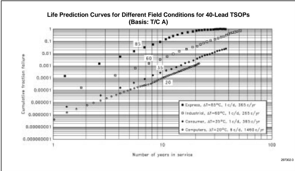
**Figure 6-3. 40-Lead TSOP Life Prediction Curves**
