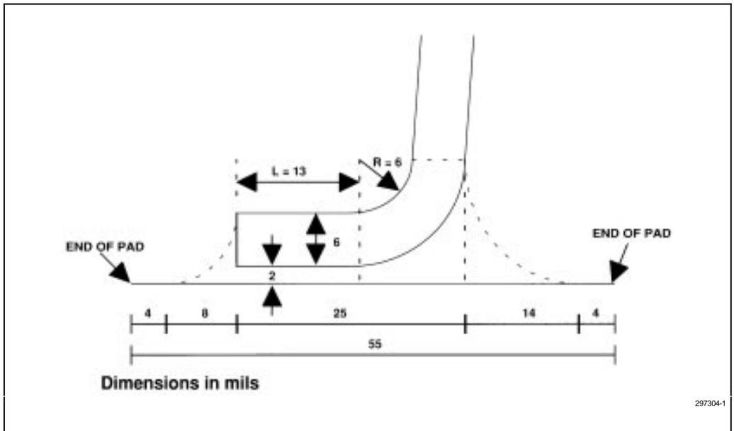
Figure 8-1. TSOP Lead Placement Close-Up View
