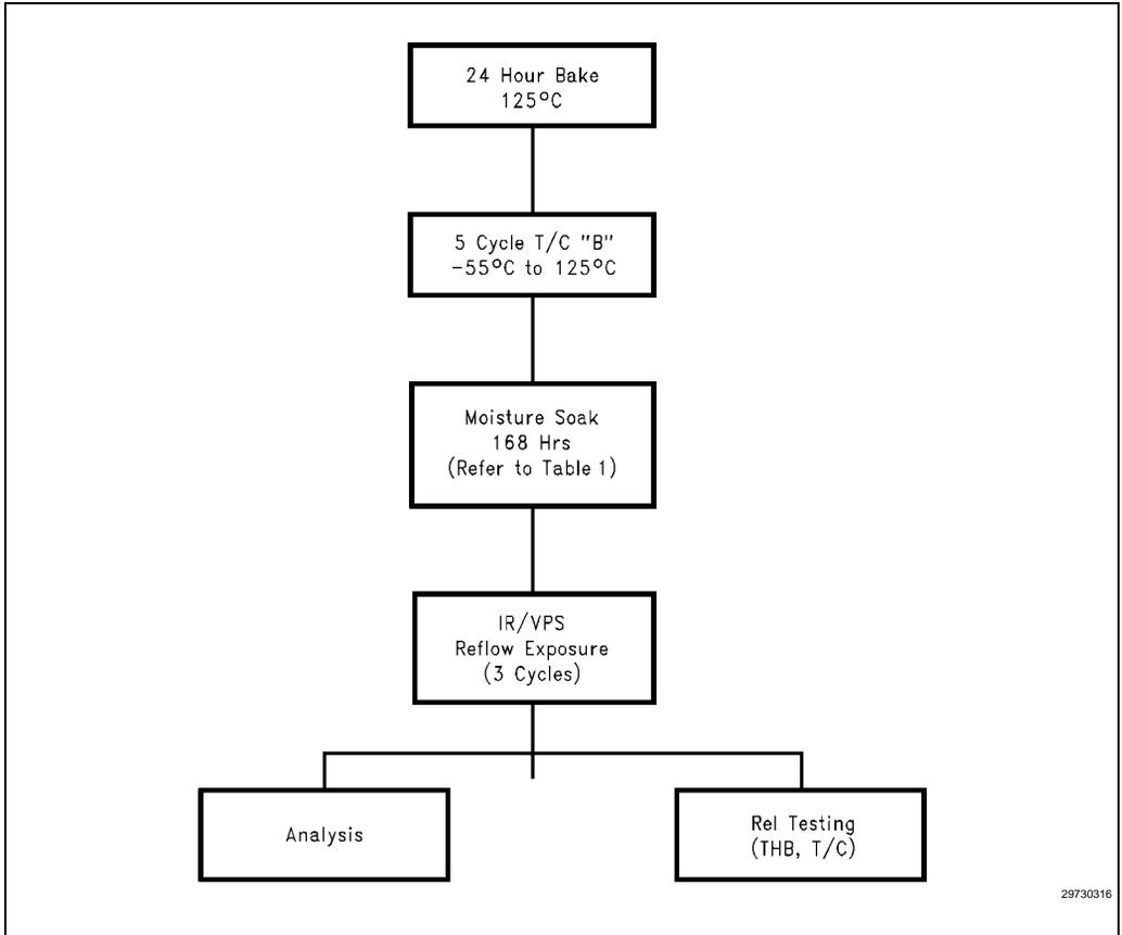
**Figure 7-13. SOP Stress Process Flow**
