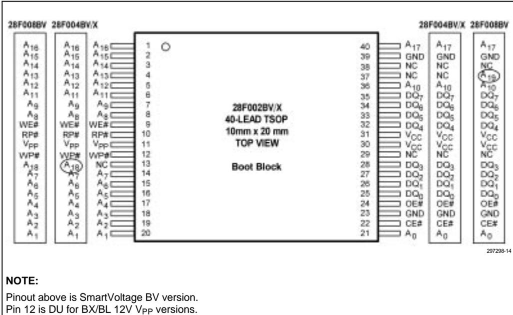
**Figure 2-5. The 40-Lead TSOP Pinout for 28F002BV and BX, 28F004BV and BX, and 28F008BV**
