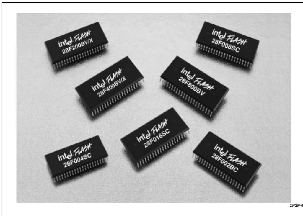
**Figure 1-6. 44-Lead PSOP Package**
