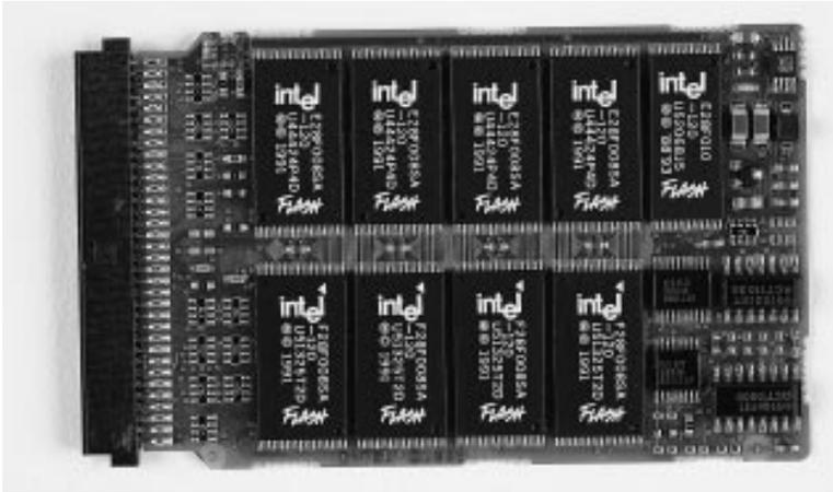
Figure 2-19. TSOP Is Ideal for Memory Card Applications
