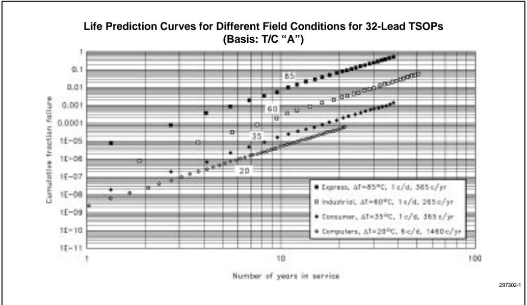
Figure 6-1. 32-Lead TSOP Life Prediction Curves
