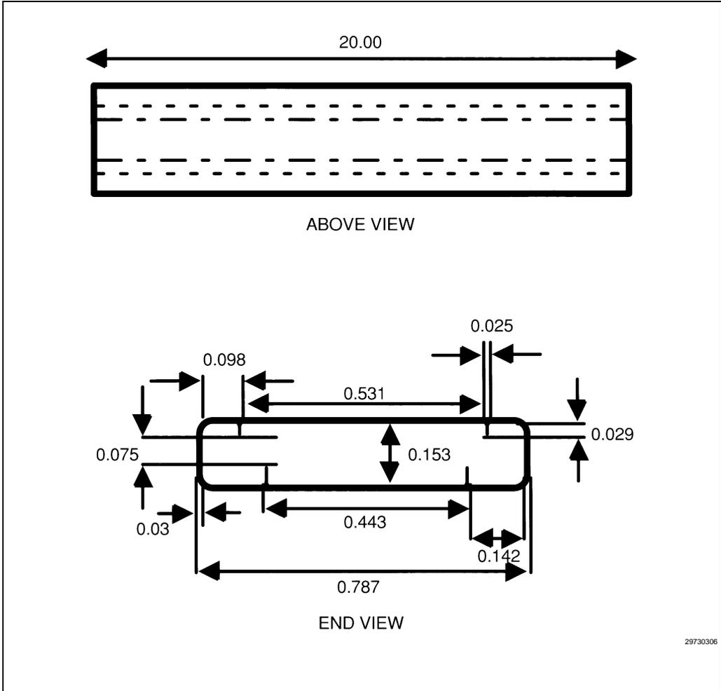
Figure 7-9. 44-Lead PSOP Shipping Tube
