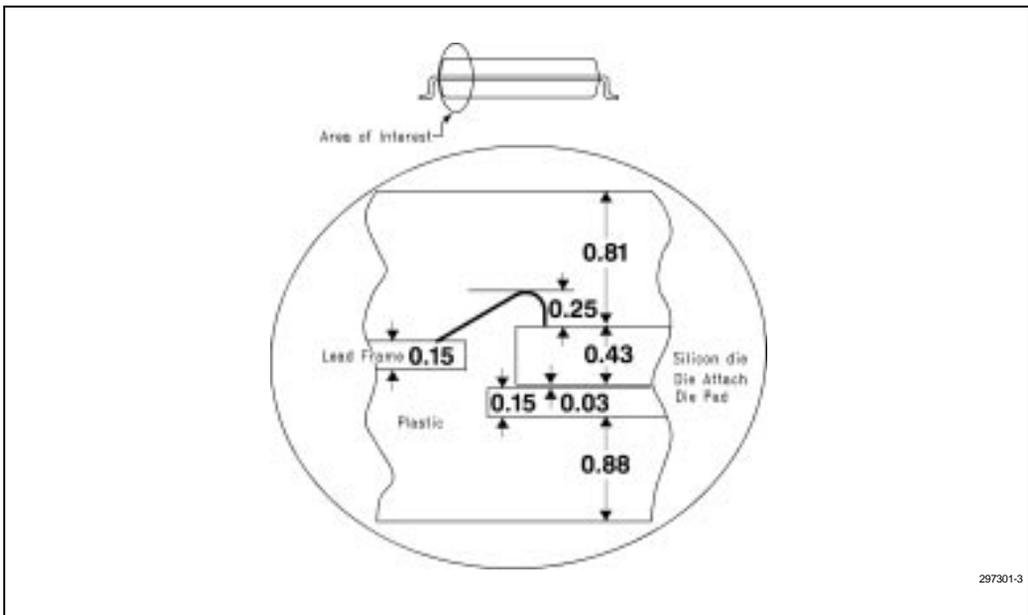
Figure 5-3. PSOP Cross Section
