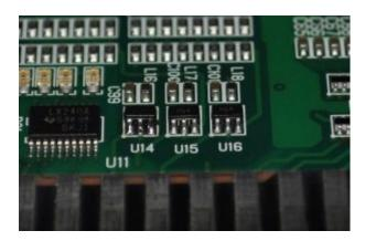
That was as good as I could get it, looks better in person but catches the flash badly. As I say you will need a fine tip iron for this as the legs are only about 0.5mm wide. Time for test mode again and checking the red output on the oscilloscope.
