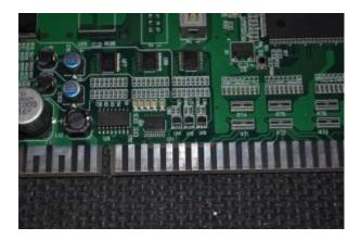
See U14, U15 and U16? Those are the colour drive amps for red, green and blue respectively. Pin 1 on the bottom left is the output, pin 3 on the bottom right is the input. These are AD8061ARTZ-\* devices, the rest of the part code is simply the packaging it's supplied in. Click here for the datasheet.
